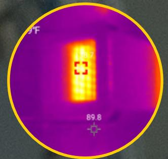
DETERMINE HOTS SPOTS IN PANELS, ON WIRING, OR ON EQUIPMENT PARTS
